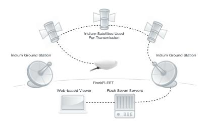
The RockFLEET allows you to track the position of your assets, and send and receive short messages from anywhere on Earth with a clear view of the sky. It can transmit using either GPRS or Iridium satellite, and works far beyond the reach of standard WiFi and GSM networks.
